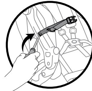
Then thread the captured screw with buckle (female) completely into anchor nut on left side of stroller accessory adapter and tighten firmly.
