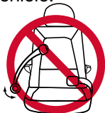
Lap belts with a sewn-in latching plate that have a retractor that locks only in case of a sudden stop.
