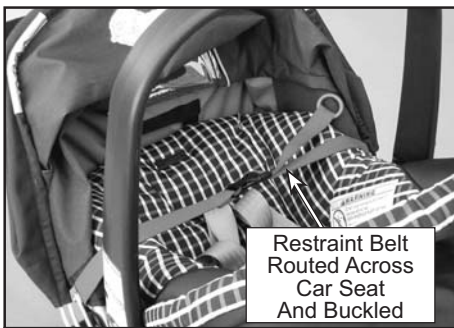
Fig. 19 Peg Perego Primo Viaggio Secured With Restraint Belt
