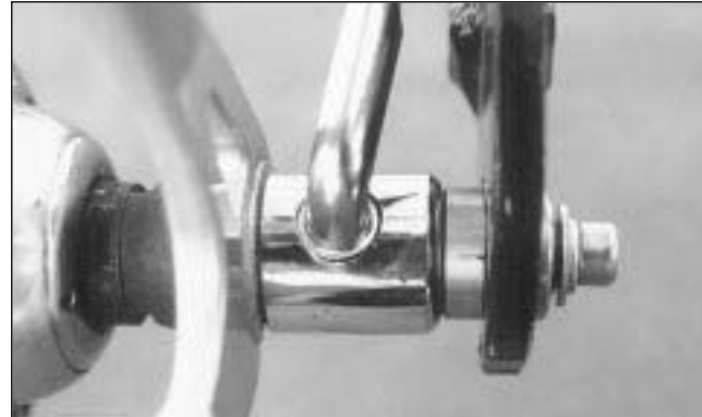
FIG. 34 Fork hooks correctly aligned and installed on bobbins.
