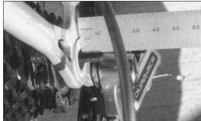
FIG. 27 Measurement of the amount of the quick release rod extending beyond the face of the dropout. The quick release must be in the closed position (FIG. 26).
