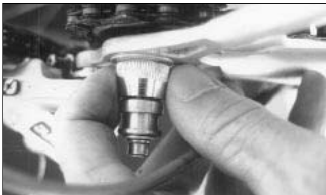
FIG. 30 Adjusting approximately 1.5mm dropout.
