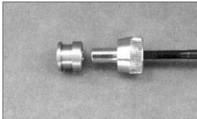
FIG. 31 Asymmetrical quick release bobbin.
