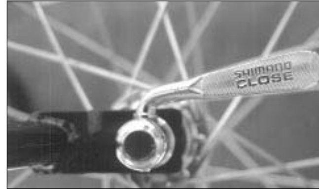
FIG. 16 Quick release in closed position.
