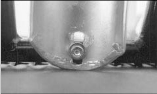
FIG. 10 Attachment of fender to trailer frame.
