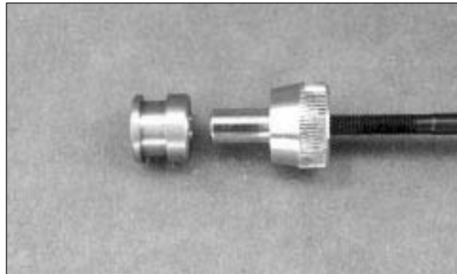
FIG. 31 Asymmetrical quick release bobbin.
