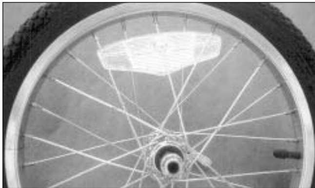
FIG. 17 Wheel reflector correctly positioned.
