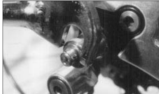
FIG. 33 Bobbin spacing does not align with hook spacing. Bobbins must be reversed for proper alignment.
