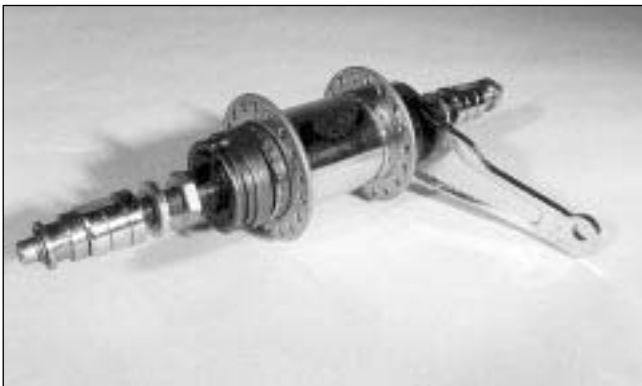
FIG. 2 BOB NUTZ solid axle adapters for bikes with solid axle hubs (includes Internal Gear Hubs).
