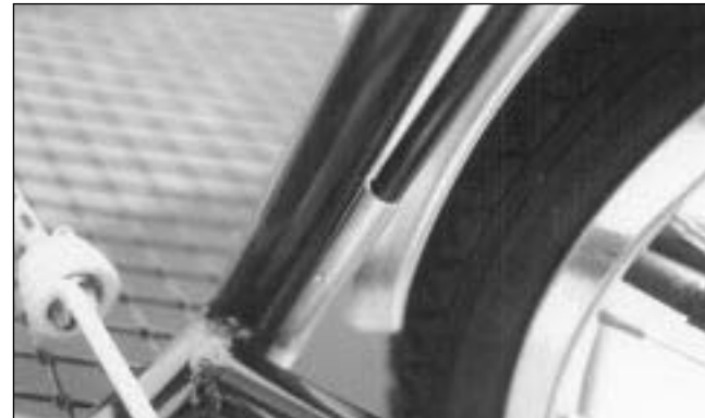
FIG. 20 YAK Safety Flag Pole installed in mounting bracket.
