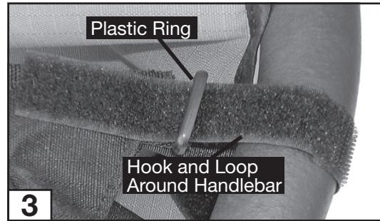
**3.** Loop the hook and loop strap through the ring and secure (Fig. 4). Repeat above steps with the front strap on the opposite side.
