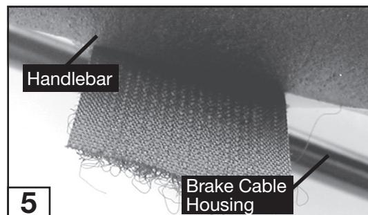
**5.** Continue wrapping the hook and loop strap around the handlebar and insert through the black plastic ring (Fig. 3).
